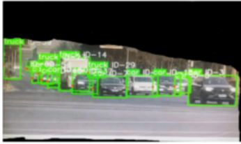
Fig. 11. Vehicle and detection datasets using fine-tuned YOLO-v5
