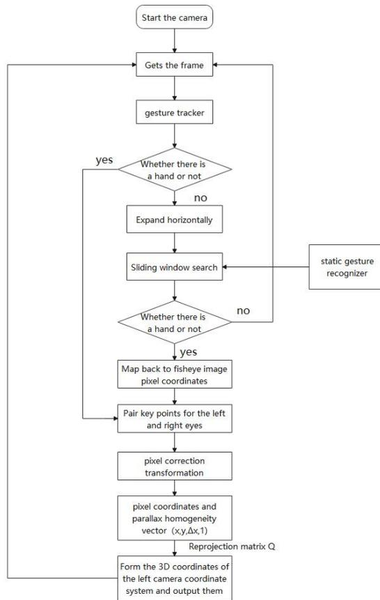
Figure 9. Flow chart of binocular fisheye gesture recognition algorithm
