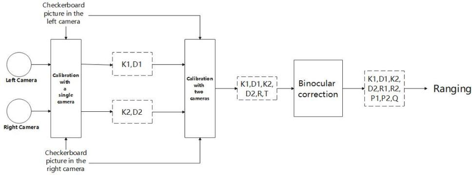
Figure 2. Binocular calibration process
