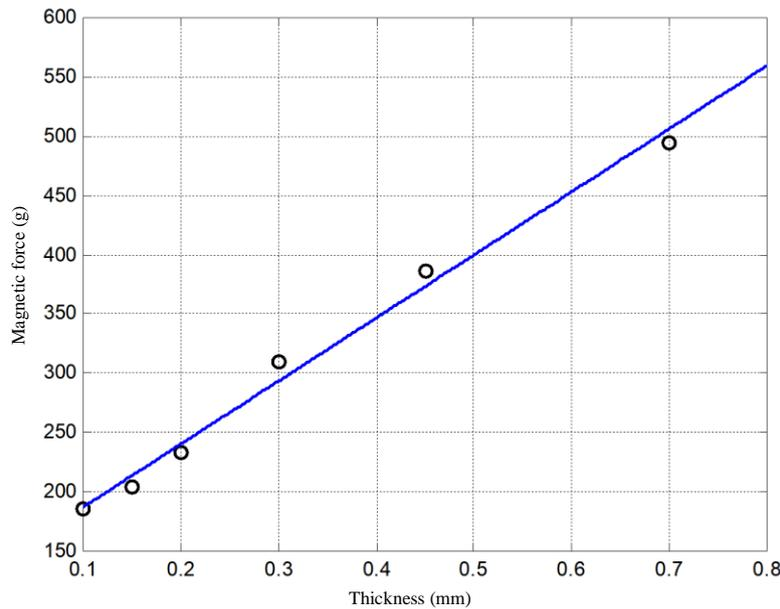
Fig.2 Relation between the magnetic forces and the coating thicknesses of the samples with titanium alloy substrate coatings
