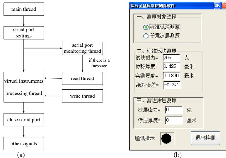
Fig.6 Serial port operation flow and interface of the thickness measurement software for coatings
