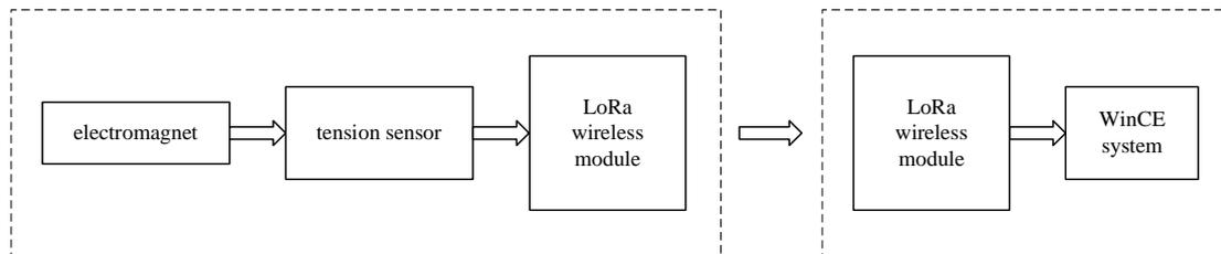
Fig.3 Block diagram of the wireless sensor system of the thickness measurement for radar absorbing coatings
