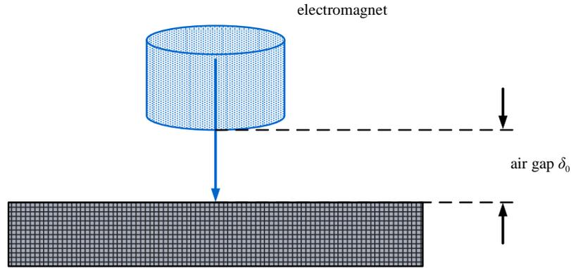
Fig.1 Model of the magnetic force between an electromagnet and a radar absorbing coating
