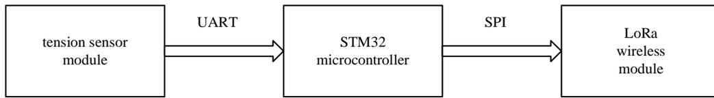
Fig 4. Block diagram of the LoRa wireless module
